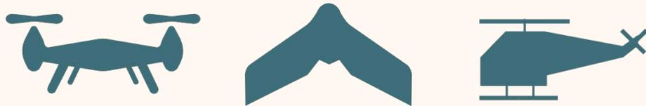
RPA can be multirotor, fixed wing, single rotor, or combinations of those designs. Each type has their pros and cons and tend to be suited to particular applications or jobs.
